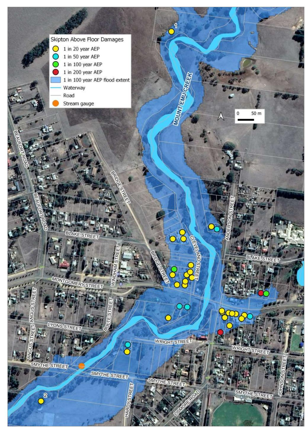
Figure 21. Skipton buildings impacted by over floor flooding for a range of design flood events (Water Technology 2020).
