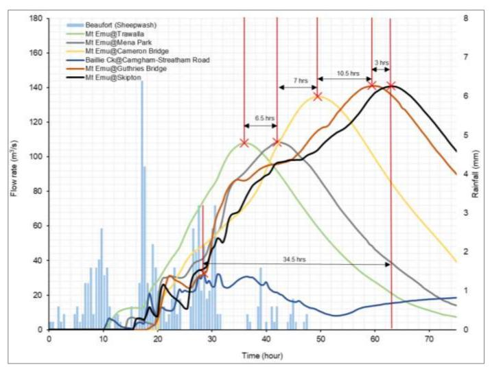
Figure 17. The travel time of flood peaks during the September 2016 flood event (Water Technology 2020).
