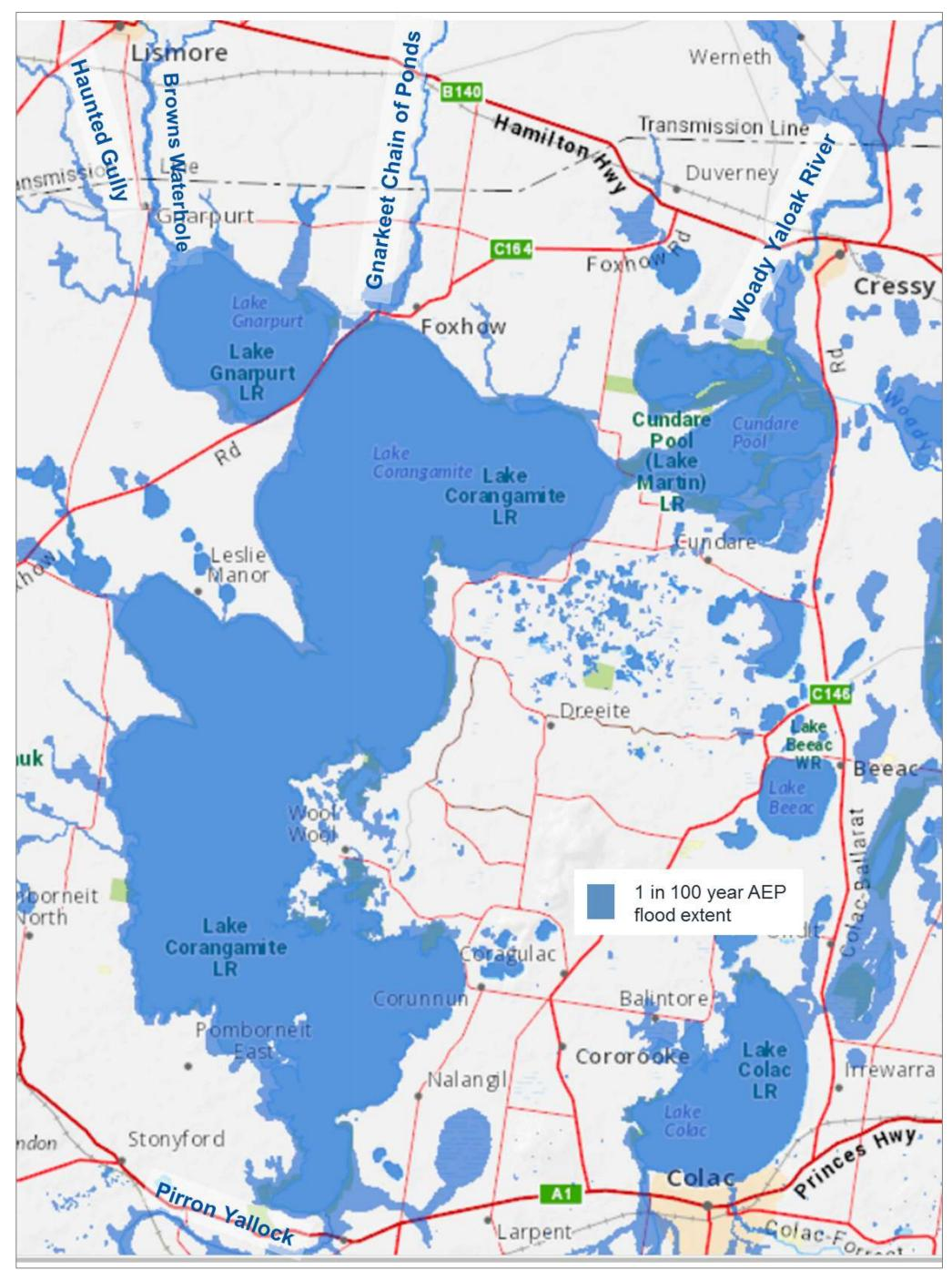
Figure 40. Flooding at Lake Corangamite during 1956 flood event, 1 in 100 year AEP flood extent (DNRE 2000).
