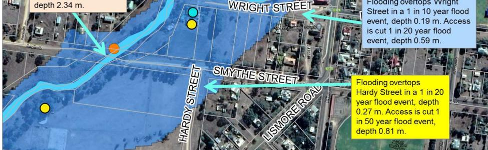
Figure 24. Skipton roads impacted by flooding with the 1 in 100 year flood extent (Water Technology 2020).
