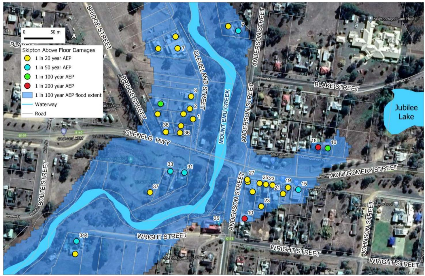
Figure 22. Skipton buildings impacted by over floor flooding for a range of design flood events (Water Technology 2020).
