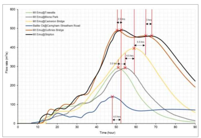
Figure 18. The travel time of flood peaks for a 1 in 100 year AEP flood, with a 48 hour duration (Water Technology 2020).
