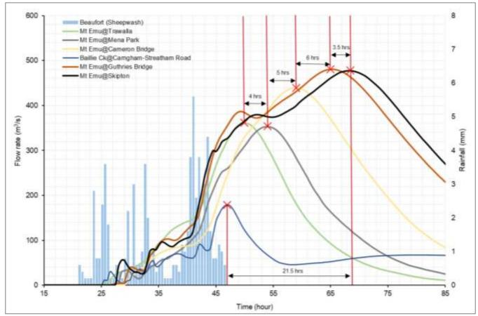
Figure 16. The travel time of flood peaks during the January 2011 flood event (Water Technology 2020).
