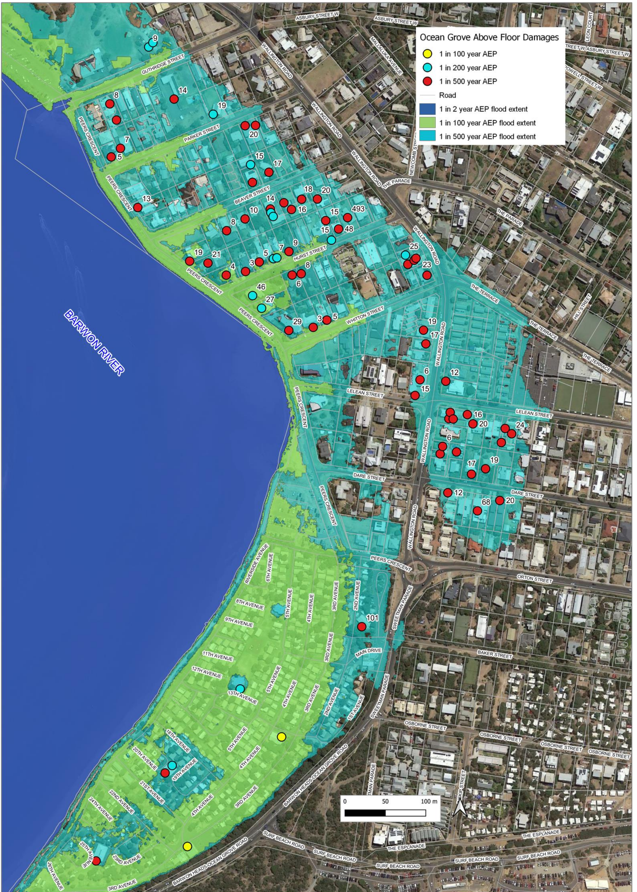
Figure 107. Ocean Grove buildings impacted by over floor flooding for a range of design flood events (Water Technology 2019).
