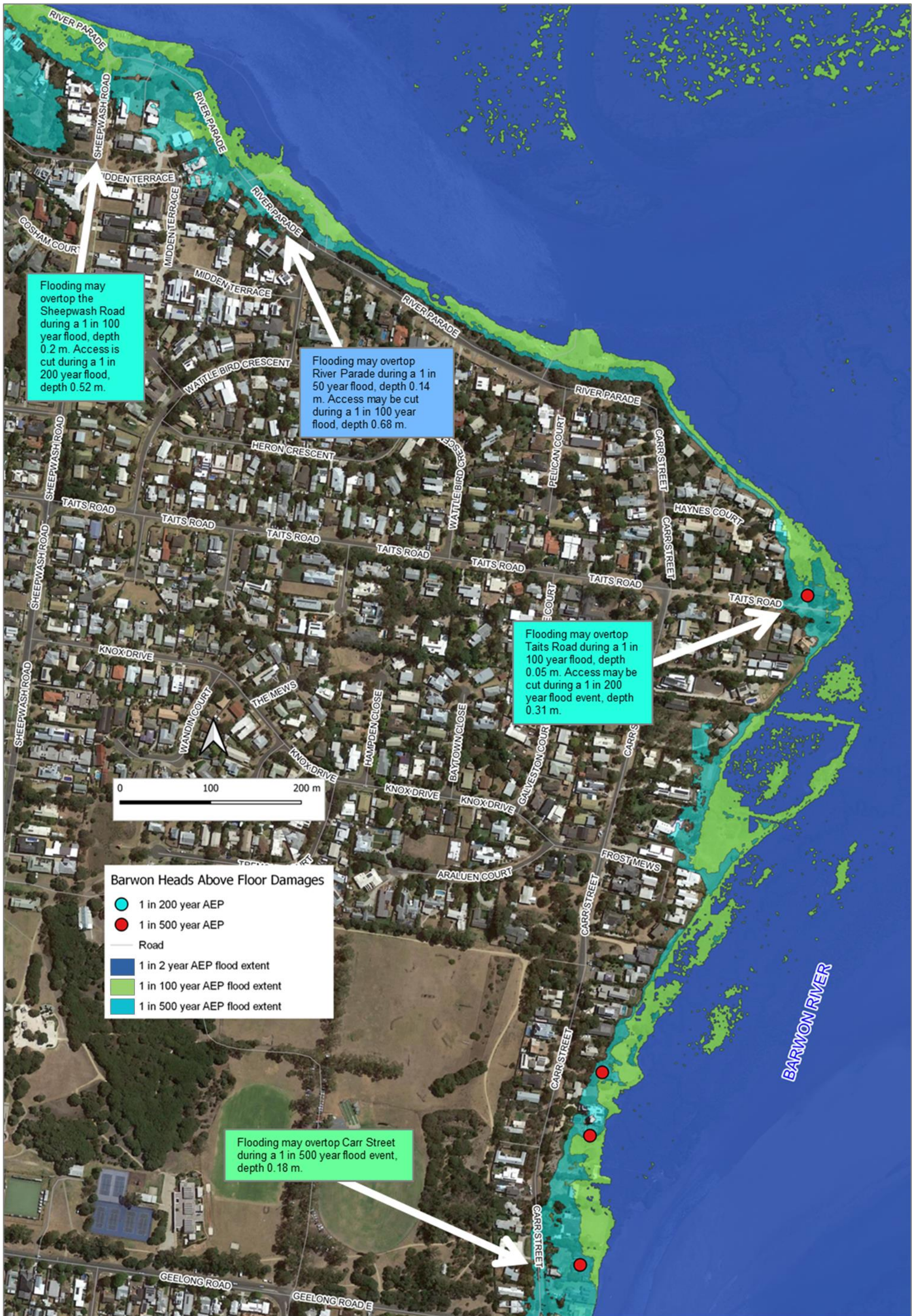
Figure 106. Barwon Heads roads impacted by over floor flooding for a range of design flood events (Water Technology 2019).
