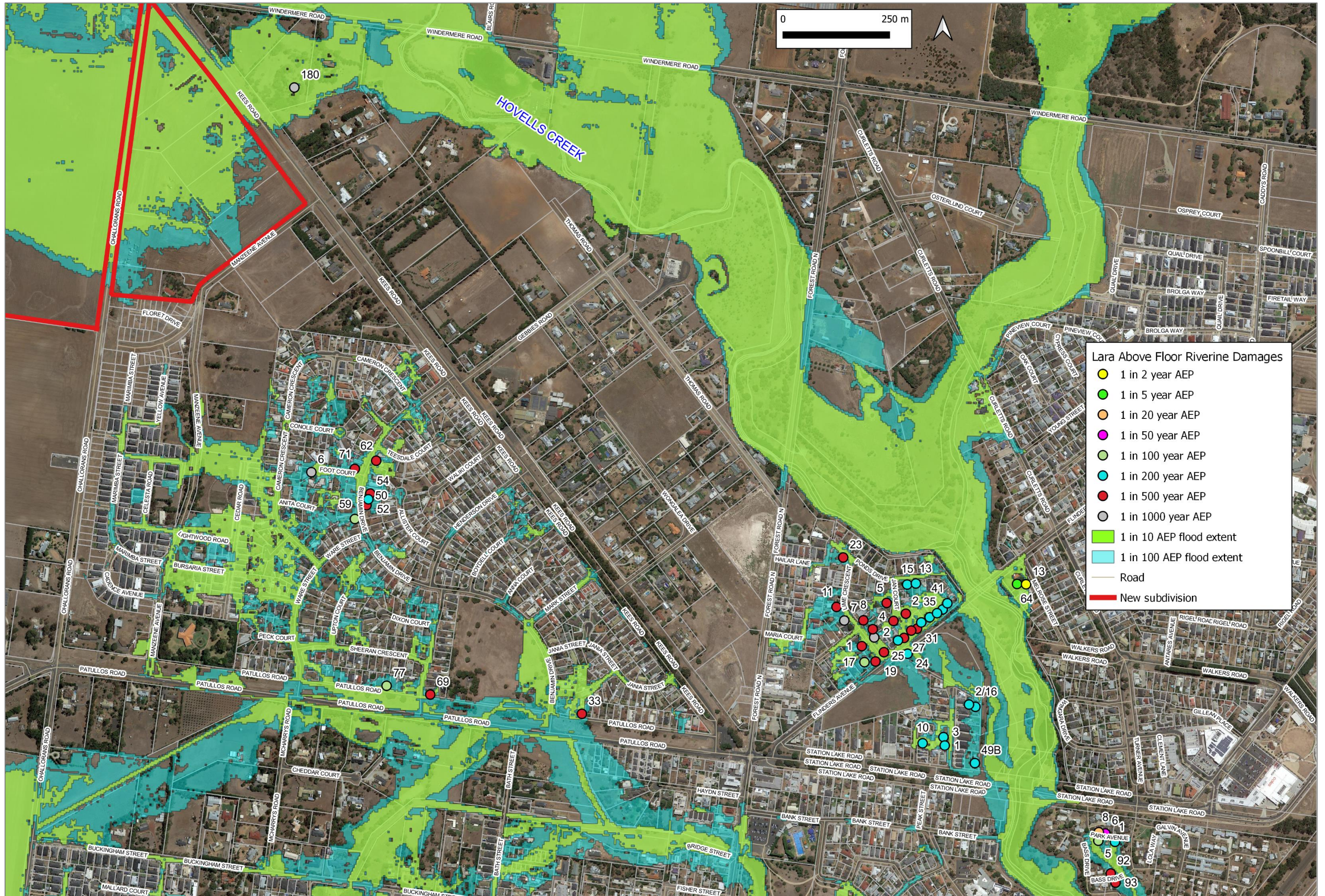
Figure 41. Lara buildings impacted by riverine flooding for a range of design flood events (Water Technology 2020).
