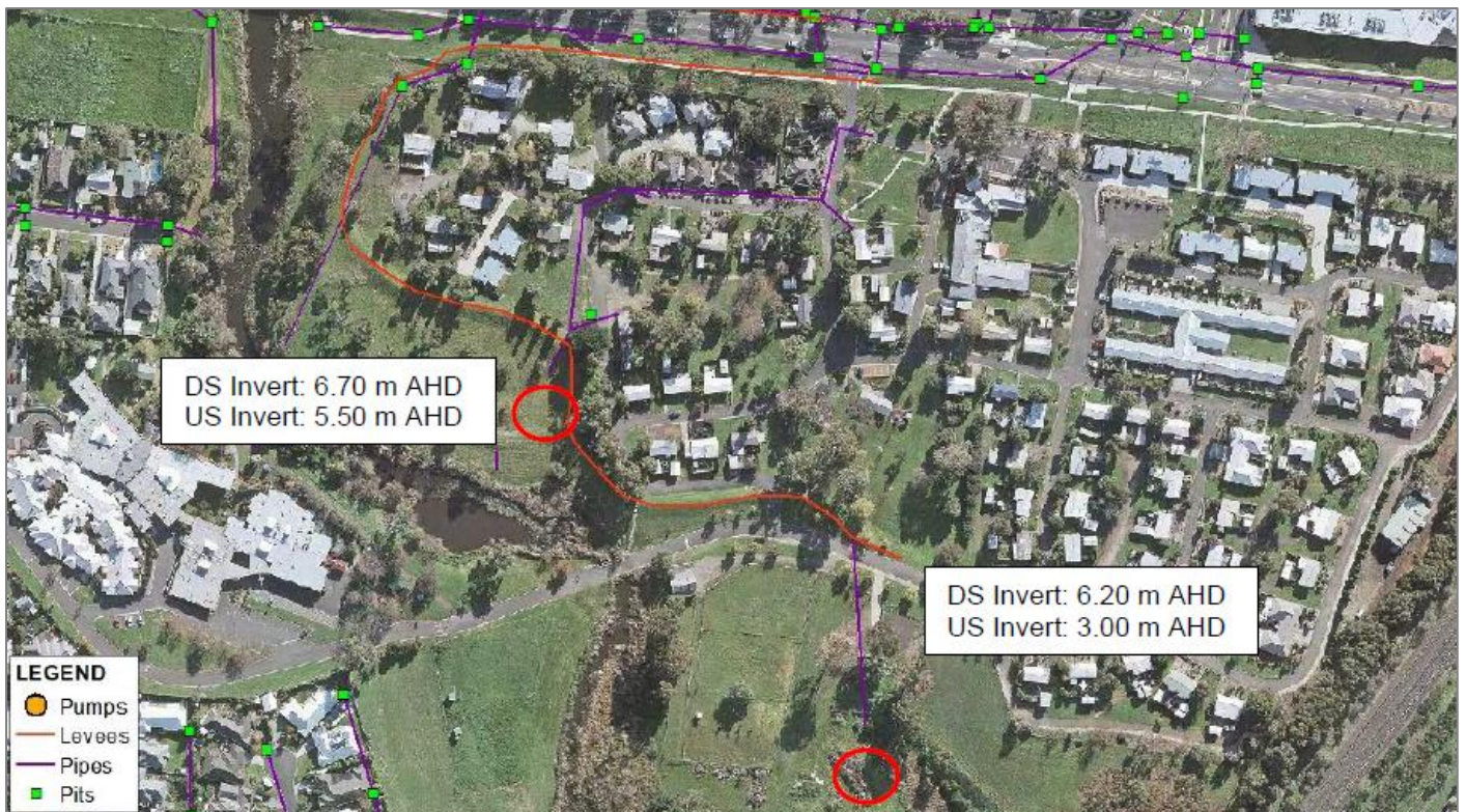
Figure 36. St Laurence Park Retirement Village stormwater drain outfall (Water Technology 2019).
