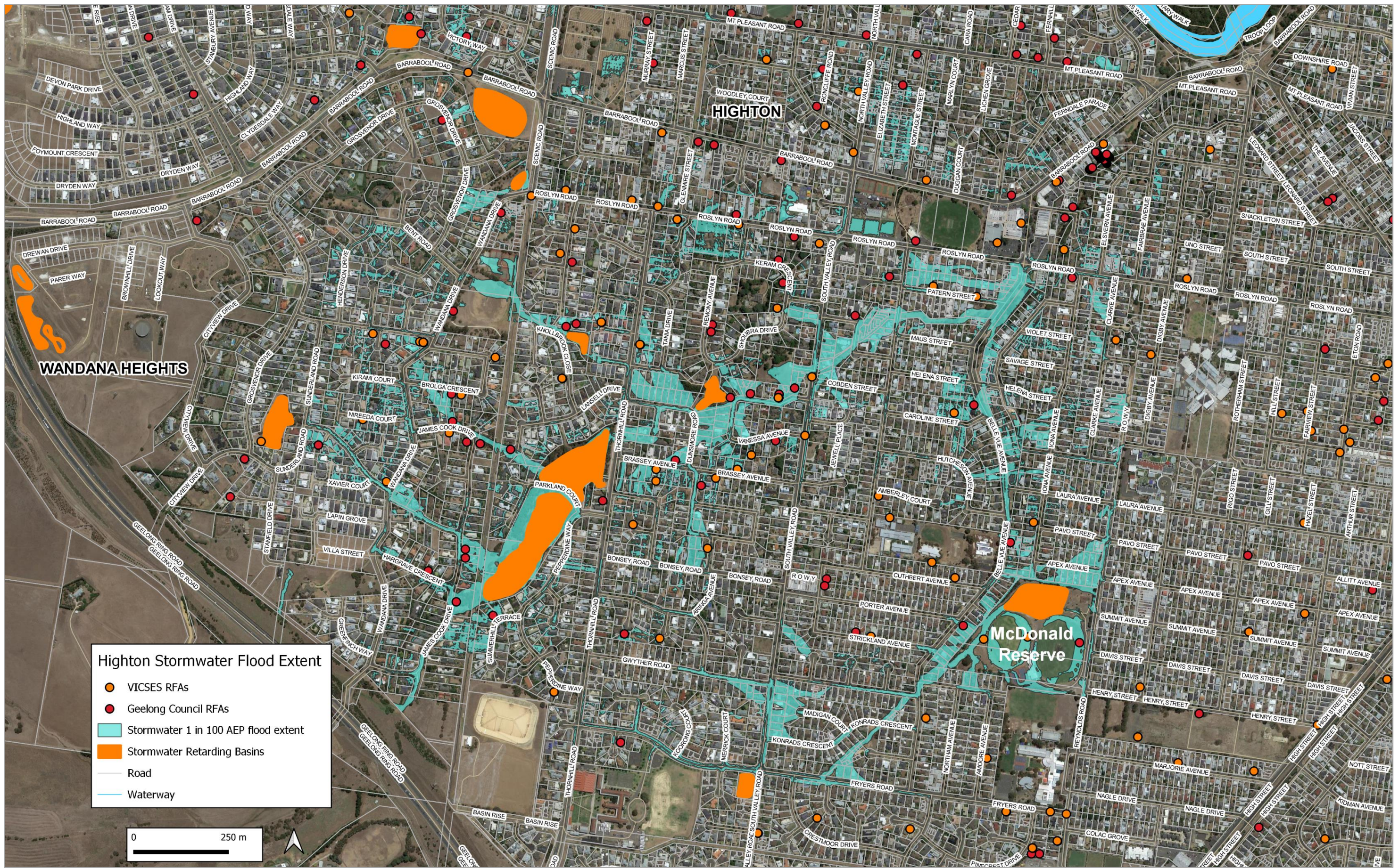
Figure 119. The Highton area in Geelong impacted by stormwater flooding, 1 in 100 year AEP flood extent (COGG 2021).
