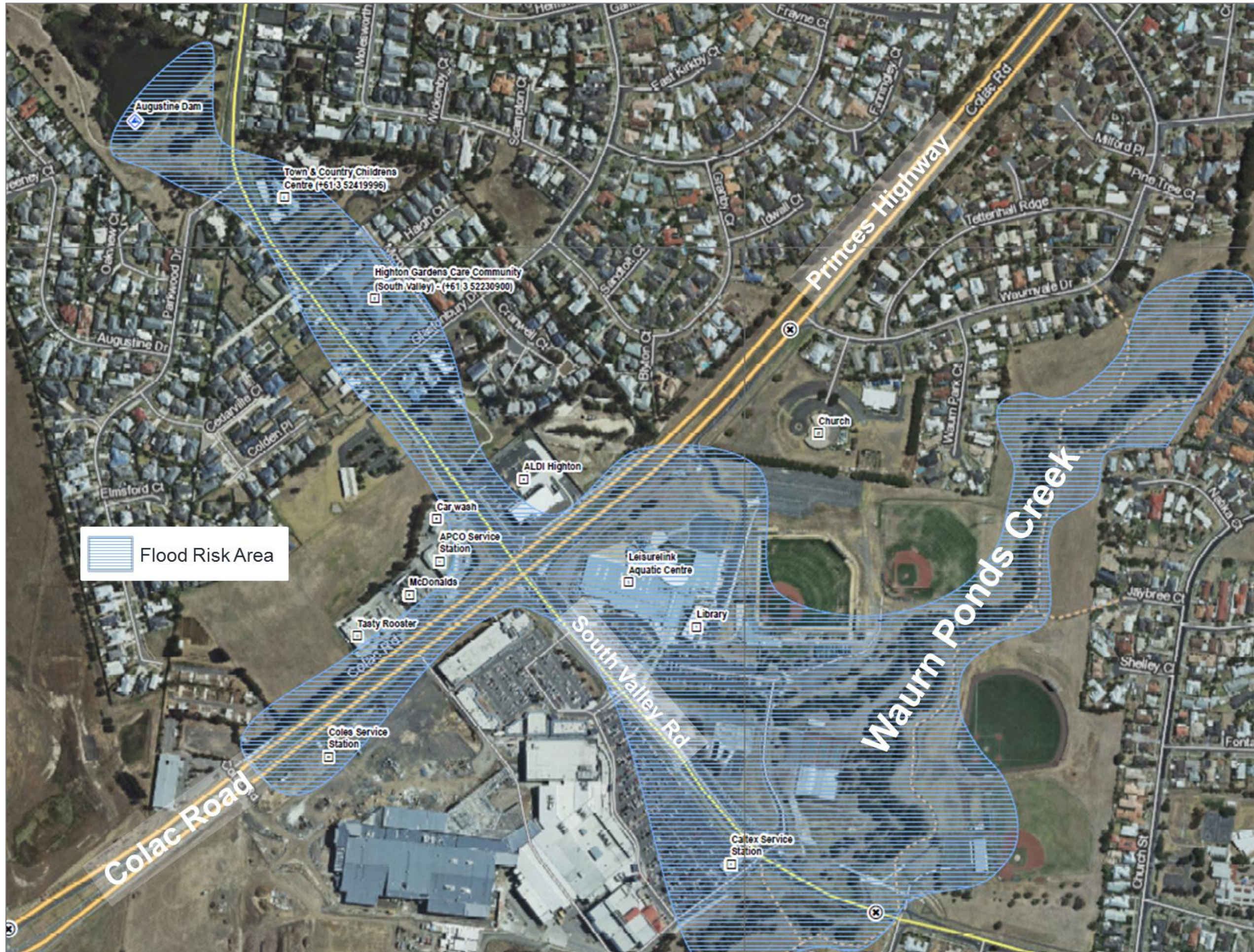
Figure 16. Failure of the Augustine Retarding Basin dam wall downstream flood risk area (DELWP 2018).
