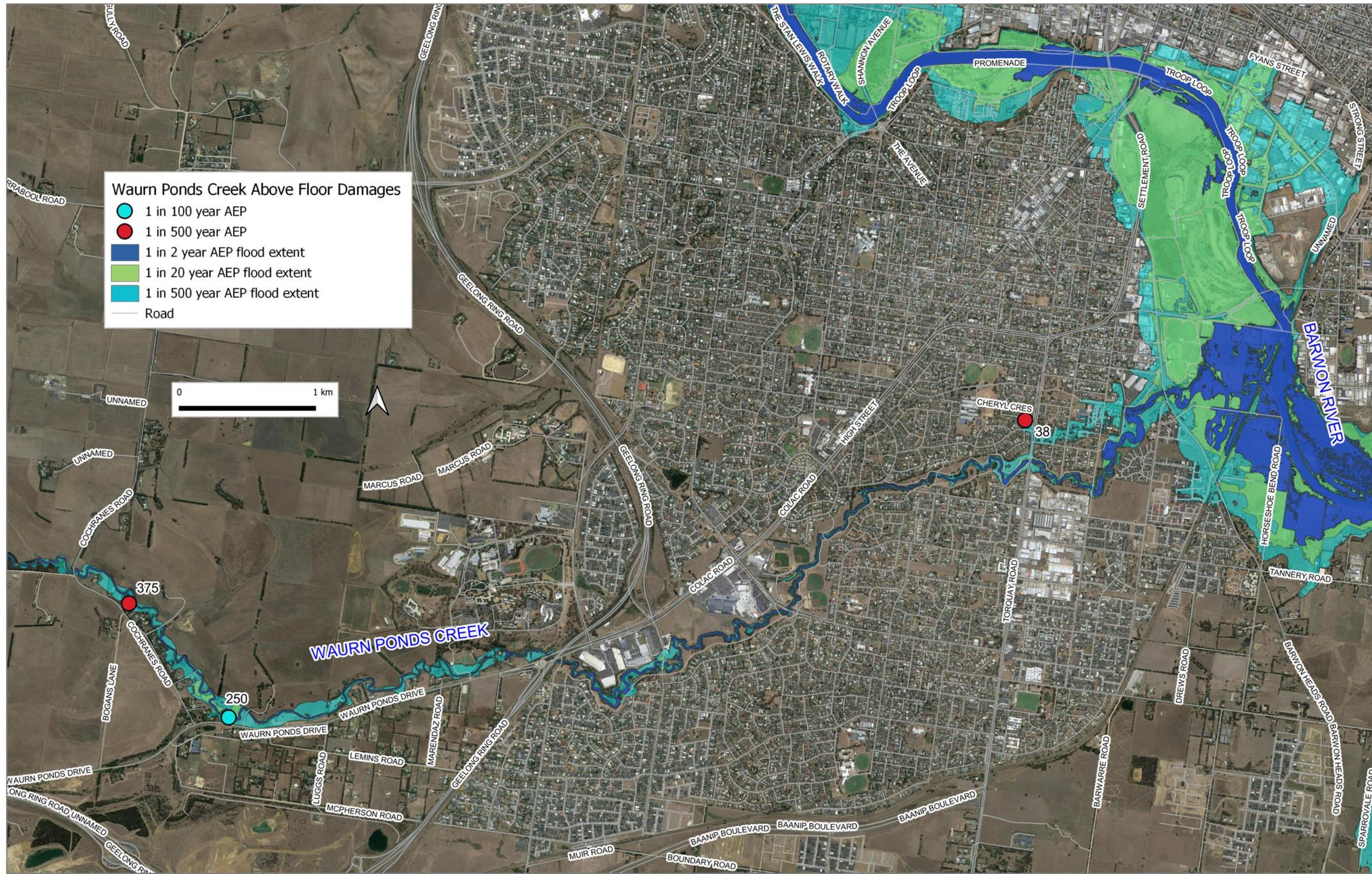
4.51 Figure 111. Waurn Ponds Creek catchment buildings impacted by flooding for a range of design flood events (Water Technology 2019).
