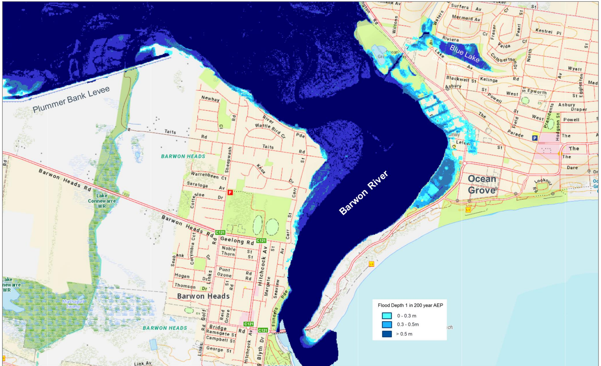
Barwon Heads and Ocean Grove 1 in 200 year AEP flood depth map (Water Technology 2019).
