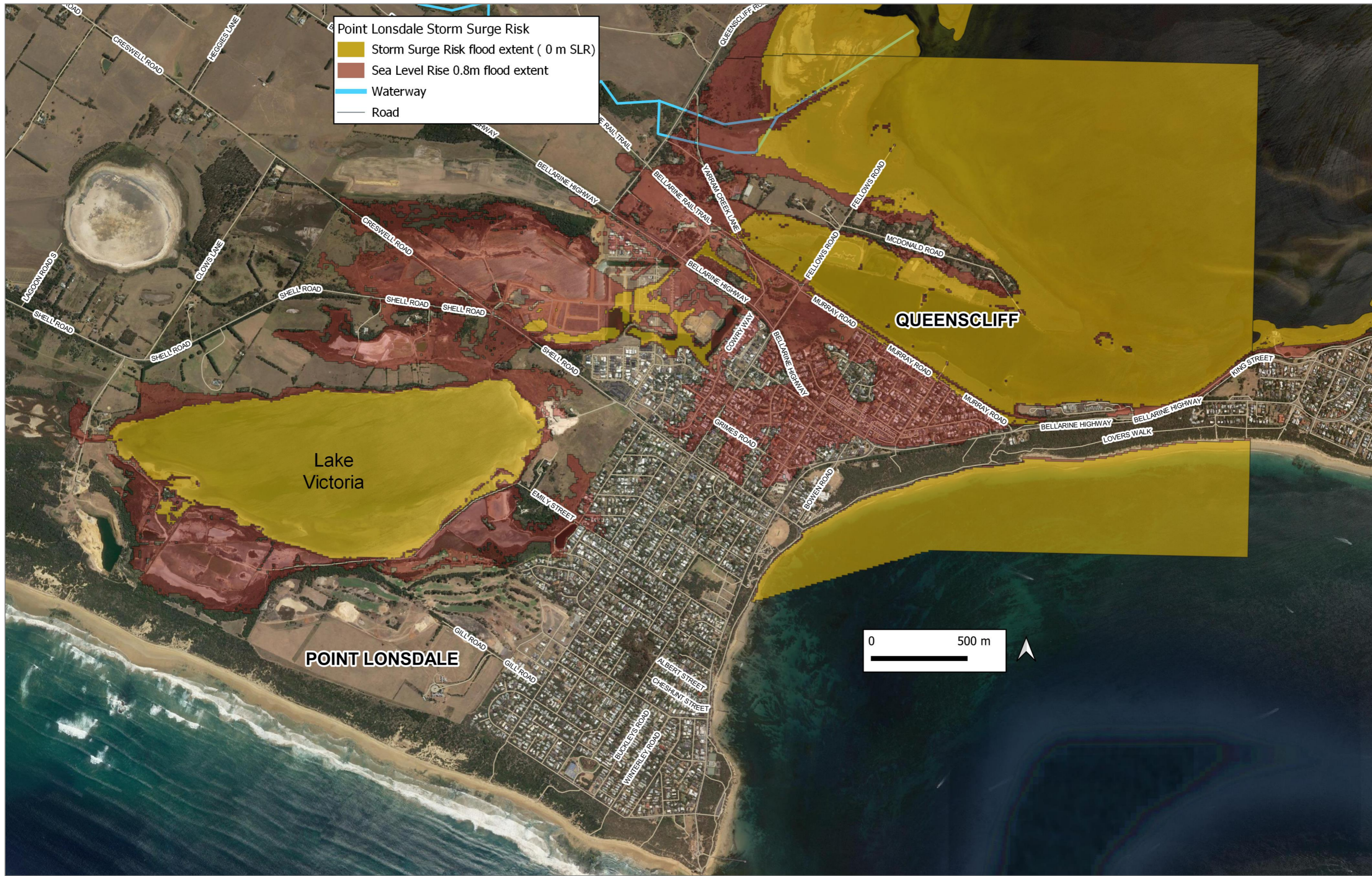
4.15 Figure 5. Pont Lonsdale storm surge (0 m sea level rise) and sea level rise (0.8m) risk flood extent (DELWP 2015).
