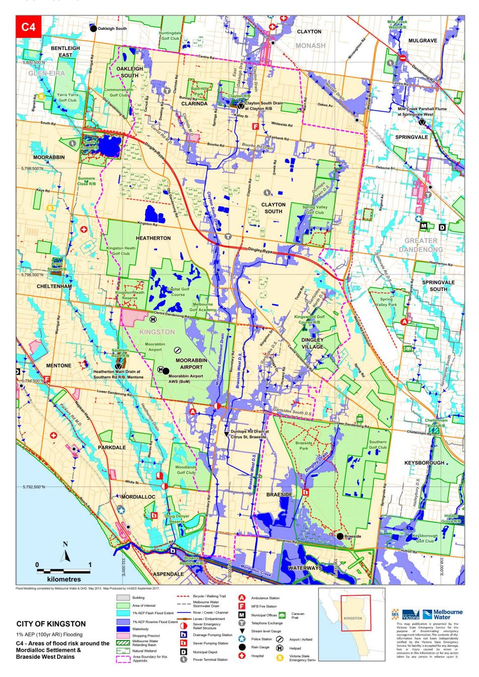
Figure C4 – Areas of flood risk around the Mordialloc Settlement Drain in the City of Kingston
