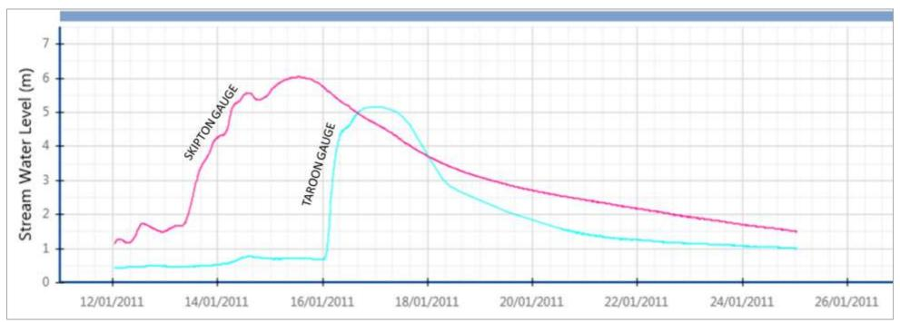
Figure 2. Panmure: Mount Emu Creek peak flows for the January 2011 flood event at the Skipton and Taroon stream gauges.
