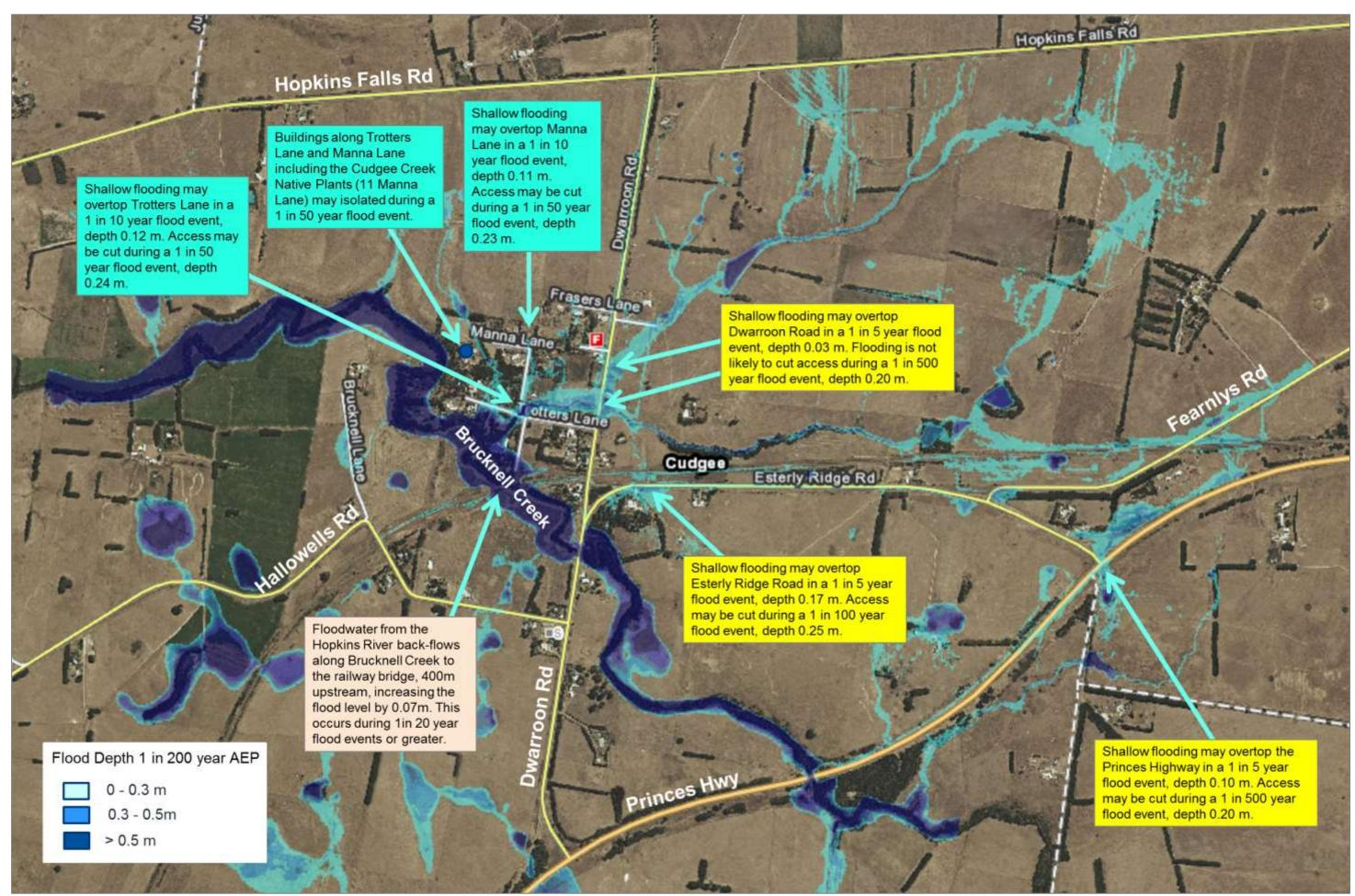
Figure 69. Cudgee roads and assets impacted by flooding for a range of design flood events (BMT 2018).
