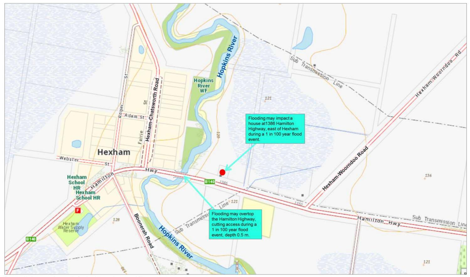
Figure 81. Hexham assets impacted by flooding during a 1 in 100 year AEP event.
