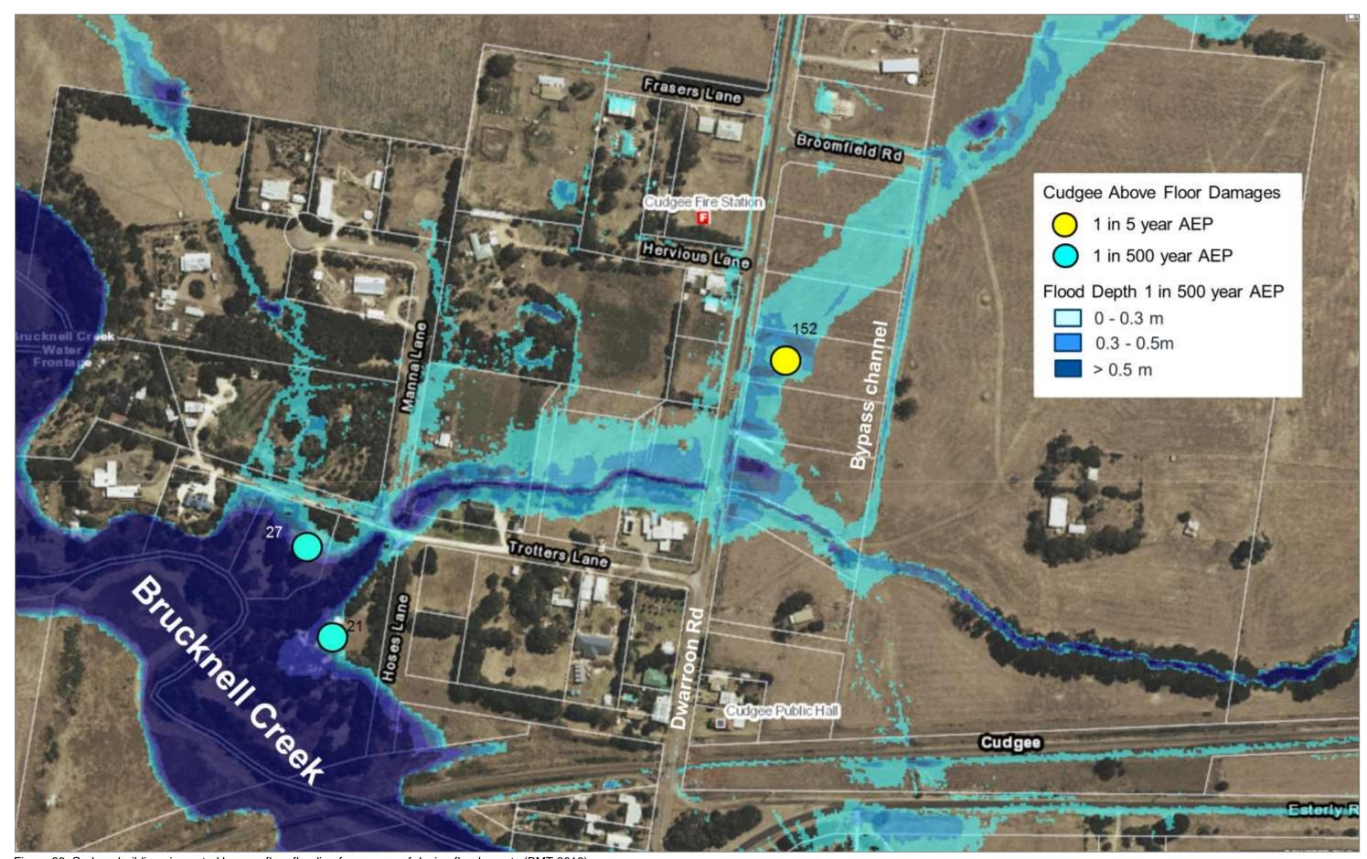
Figure 68. Cudgee buildings impacted by over floor flooding for a range of design flood events (BMT 2018).
